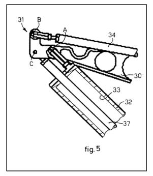
line 1 and line AC is always parallel to line 2 due to the presence of the first and second parallelograms, while angle BAC defines the angle between the imaginary lines 1 and 2. As the manipulator 14 is still free to move in a circle around the toggle lever 31, the spatial position of the manipulator 14 is determined by the rotor of the second motor means 23 and the second movement unit 26.
