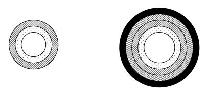
= inert sugar core particle, = methylphenidate HCl (5-20% w/w)+ binder such as HPMC (0.5-5% w/w) = seal coat (up to 4% w/w) = dissolution rate controlling polymeric coating = seal coat (up to 4% w/w).
