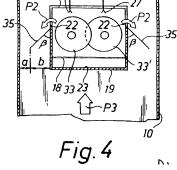
In the board's view, the structural means of the device defined in claim 13 of the main request can be read in the following means of the device illustrated in the above Figures: - the "contact reactor through which the process gases are intended to be passed" corresponds to the space between the duct (10) and the box materialised by the bottom (19) and top (20); see also arrow P3 which shows the flow of the flue gas containing the gaseous pollutants
