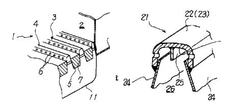
equipped with injection holes 6, and the valley parts 5 being composed of a refractory material 7. According to the abstract, the purpose of this design was "to
