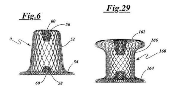
The Board considers it important to clarify that in the context of the present invention, as also acknowledged by the appellant, the word "shoulder" designates the surface of the radially expanded part directly following the body portion (the parts referenced 54 or 164 in the two drawings above) and not the base surface at the very end of the device ("flat" surface in the two embodiments shown).
