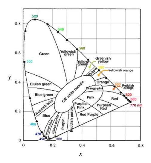
2.2 It is well known that if two colours are represented with their x,y coordinates as two points on the 1931 CIE Chromaticity Diagram and these points are joined by a straight line (segment), all the colours corresponding to the x,y coordinates of the points of this segment can be reproduced by mixing the two colours defining the two end points of the segment.
