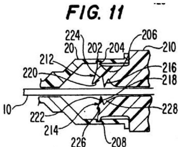
In this embodiment a "distal end cap 210 includes a pair of needle jaws 212 and 214 which have flexible pincers 216, 218 with contact surfaces 220, 222 formed as intermeshing, complementary, saw-tooth surfaces. Included in the saw-tooth surfaces are latch locks 224
