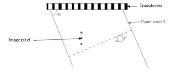
In contrast to conventional techniques where the raw data thus obtained are used to calculate image pixels, the method according to the invention repeats the transmission steps for a plurality of propagation directions  $\alpha_i$ .
