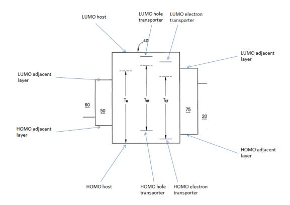
As can be seen in this figure, the energy gap between the HOMO and LUMO of the host (the two horizontal lines of the perimeter of box 40) is greater than the corresponding gaps of the electron and hole transporting materials (horizontal solid lines in the middle and right-hand part of box 40). Hence, the first condition of claims 1 and 2 is fulfilled.
