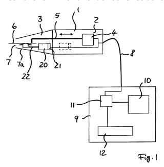
Moreover, paragraph [0013] discloses that, in one embodiment, the storing chamber also comprises an inlet ("Öffnung") provided with a vent valve ("Lüftungsventil"). As in the contested patent, the inlet lets air from outside enter the storing chamber to compensate for depletion of the staining solution during the process of tattooing ("Öffnung zum Nachführen von Luft beim Ausbringen des flüssigen Wirkstoffs").
