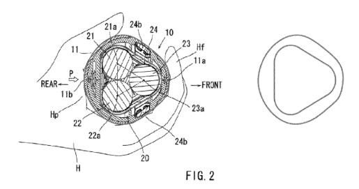
5.2.1 According to the opponents, in the example shown in figure 2, which is the only embodiment described in the patent, the cross-sections of the battery pack and of
