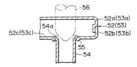
Moreover, the use of a jig (56) to deform the heat transfer tube (54) is incompatible with the microchannel construction of the heat transfer tubes of D10 (4) and D11 (12) since the work of the jig would collapse the end portions of the walls (D10: 4a; D11: 12a) defining the microchannels.
