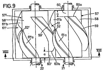
long blade 59' is formed by the axial end section 60'a. The rearward end section of the long blade 59' then lies at the opposite axial end roughly at the same axial position as the end section 60a of the long blade 59.
